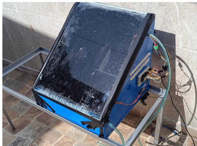
Figure 4. Final design of solar still monitoring system through IoT
